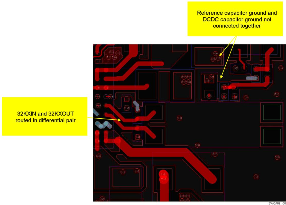
Figure 8. Reference and 32-kHz Oscillator Layout IN1
