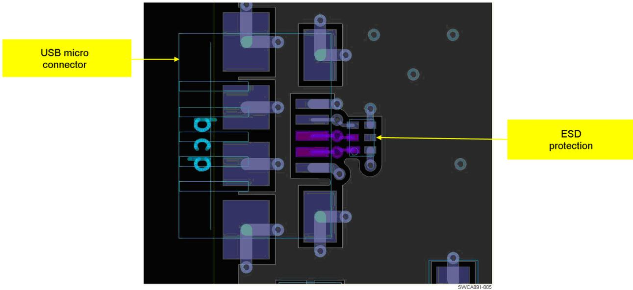
Figure 6. USB Board Layout TOP/IN1 Side
