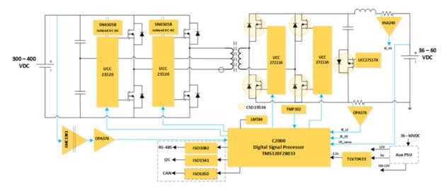
Figure 1-3. Block diagram of the isolated bi-directional DC-DC converter
