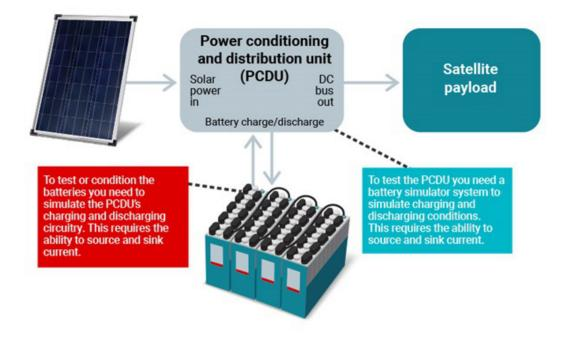
Figure 2. A typical satellite EPS
