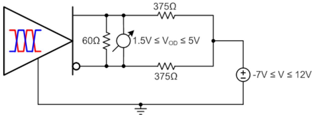
**Figure 5. RS-485 Output Driver Test Circuit over Common-mode**
