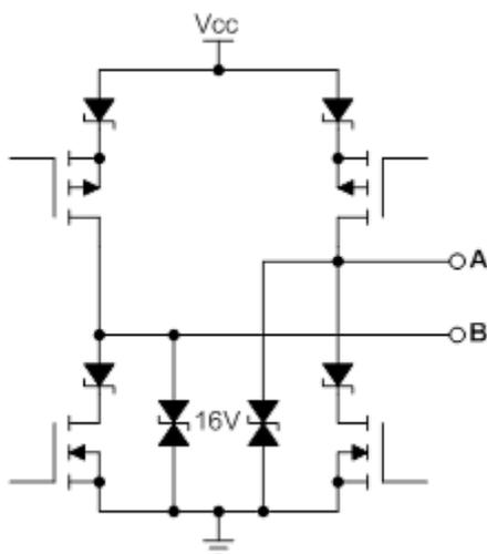
**Figure 1. Differential Output Driver Structure**
