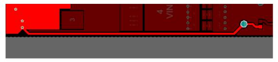
Figure 2. Feedback Trace Routed along the Edge of the Board to Avoid Noisy Switch Nodes
