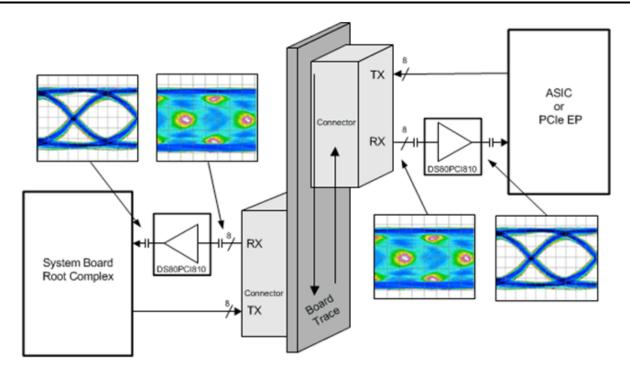
Figure 1. DS80PCI810 PCIe Gen 3 Redriver Typical Application Block Diagram
