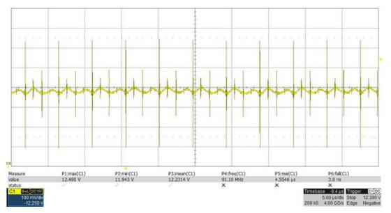
Figure 2. Output Ripple/noise 200 MHz Bandwidth in Design without Ground Plane (12V 8A off 52VIN)
