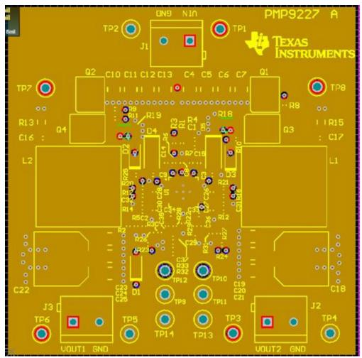
Figure 1. PMP9227 Layer 2 Ground Plane
