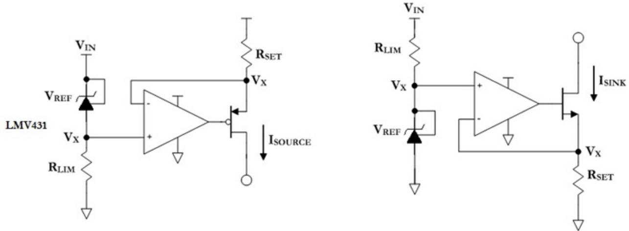
**Figure 2. Feedback-generated Current Source and Sink Circuits**
