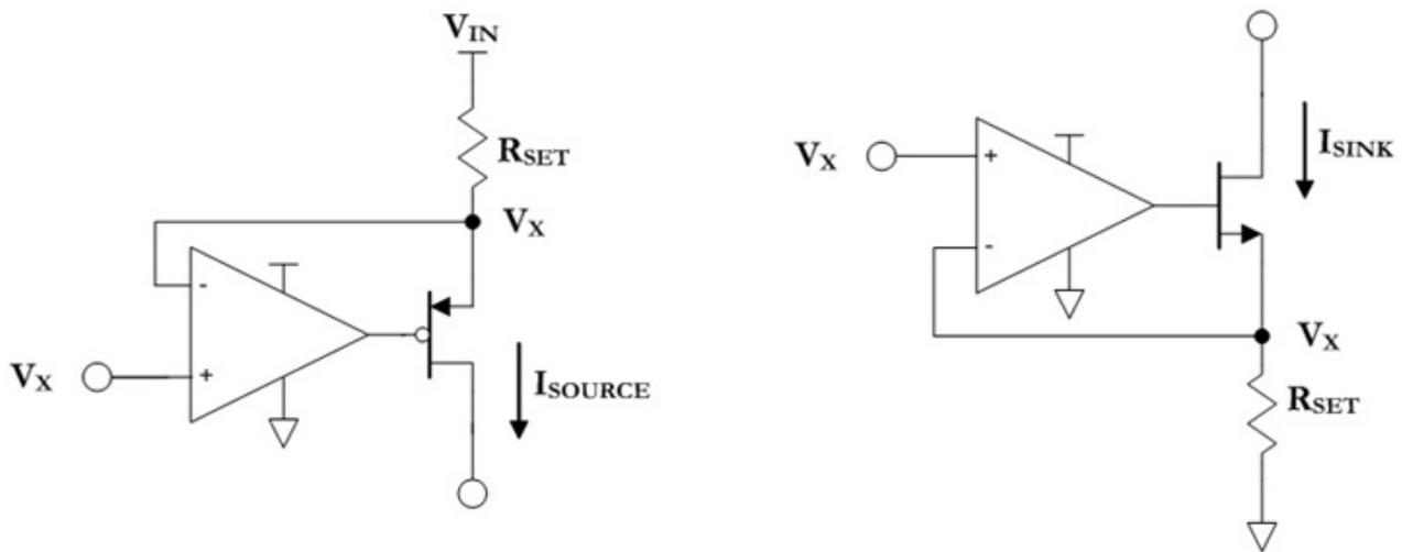
**Figure 1. Feedback-generated Current Source and Sink Circuits**
