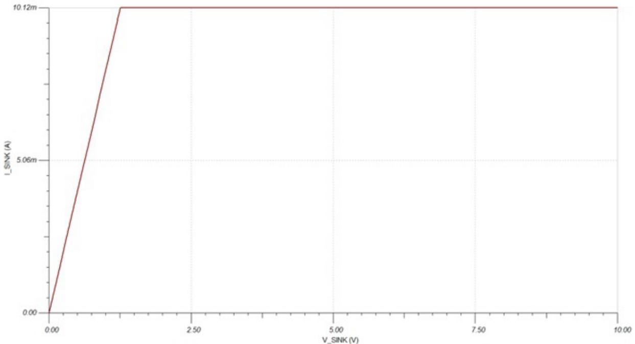
Substituting a bipolar junction transistor (BJT) for the FET in this topology may result in a marginally higher headroom requirement, although ultimately this substitution should behave almost identically.
