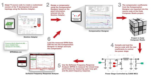
The values from the Solution Adapter GUI are used by the PFC power stage model in the Compensation Designer to plot the theoretical loop gain Bode plots for both the voltage and current loops of your custom PFC board. You can then modify the compensator values from this GUI to achieve the desired loop bandwidth, gain margin, and phase margin for both the voltage and current loops.
