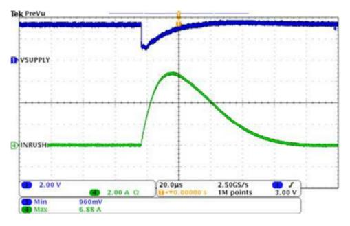
Figure 2. Power-Supply Dip Due to Inrush Current
