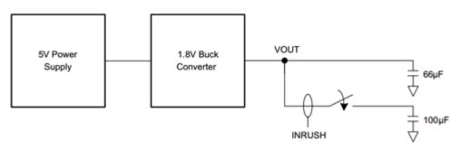
Figure 4. System Block Diagram without Slew-Rate Control
