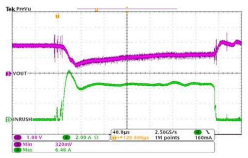
Figure 5. Inrush Current and Voltage Drop without Slew-Rate Control
