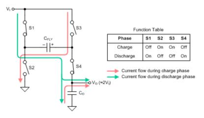
Figure 1. Simplified Charge-pump Block Diagram (Voltage Doubler)
