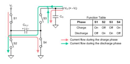
Figure 2. Simplified Charge-pump Block Diagram (Voltage Inverter)
