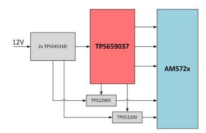
TPS659037 is a low-voltage power management IC, supporting 3.135V to 5.25V input voltage. The device offers 7 DCDC switching converters, 7 LDOs, and other power management features including SmartReflex support, 8x GPIOs, watchdog, interrupt handling, and a 12-bit GPADC.
