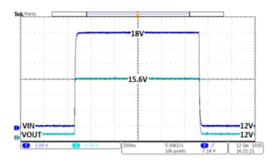
Figure 2. eFuse Output-voltage Clamping Using the TPS25924
