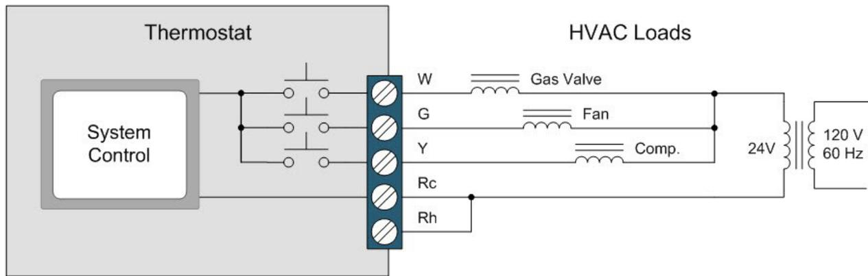
**Figure 2: Functional diagram of a basic thermostat**
