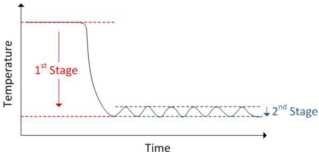
**Figure 3: Temperature vs. time for first- and second-stage cooling systems**
