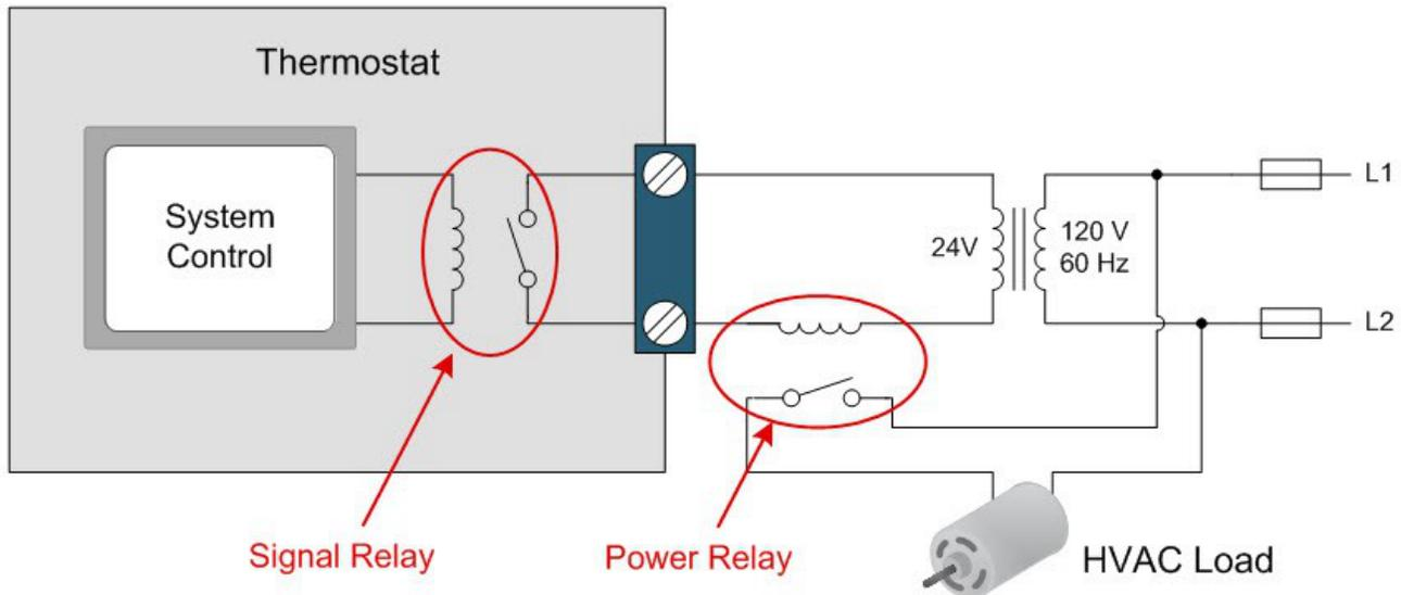
**Figure 4: Single thermostat signal-relay connection with HVAC load**
