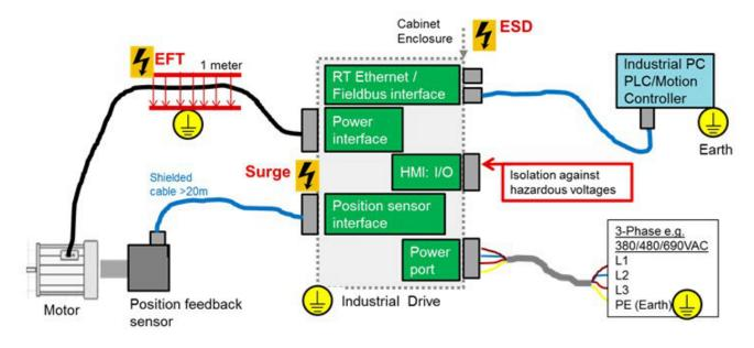
Figure 2. Example EMC Immunity Test Signals in an Industrial Drive
