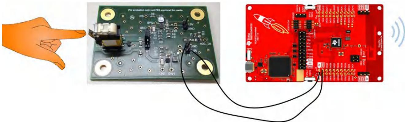
**Figure 1. Energy Harvesting for Wireless Switch Power Reference Design**
