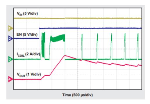
Figure 1. Because of This FPGA's High Startup Load and Very-High Decoupling Capacitance, the DC/DC Converter Cannot Bring Its Output Voltage into Regulation
