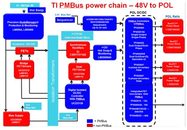
Figure 1. 48V to Point-of-load PMBus Power System
