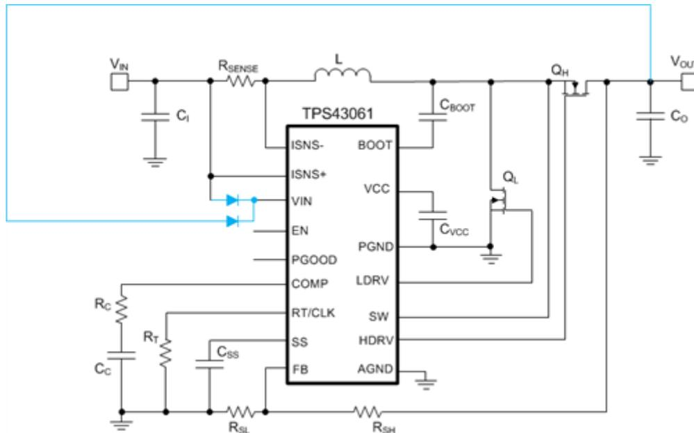
Figure 2.  $V_{IN}$  Biased from  $v_{OUT}$  Of TPS43061
