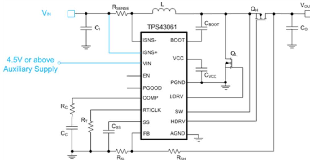
**Figure 3.  $V_{IN}$  Biased from an Additional Supply**
