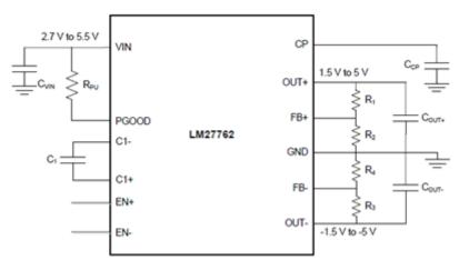
Figure 4. The LM27762 Split-rail Charge Pump with Integrated LDOs
