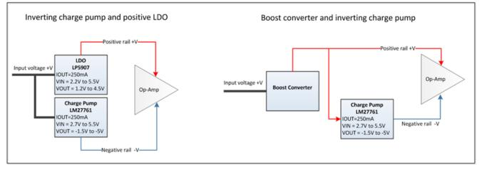
Figure 3. Split-rail Solutions Combine an Inverting Charge Pump and a Positive Voltage Regulator
