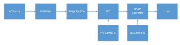
Figure 1. Discrete Controller IC-based AC/DC Design
