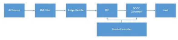
Figure 2. Combo Controller IC-based AC/DC Design
