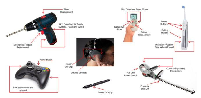
Figure 1. Grip Detection in Different Applications
