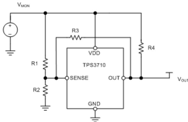
**Figure 1. TPS3710 With Resistors Added for Hysteresis**
