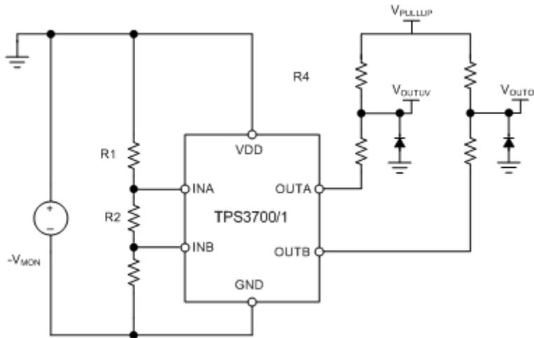
Figure 2. TPS3700/1 Configured for Negative Voltage Sensing
