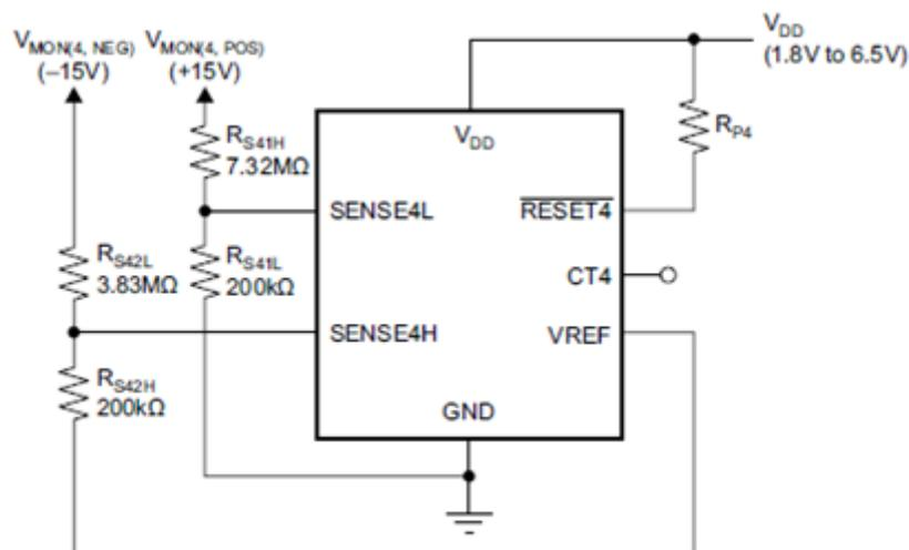
Figure 3. Using an External Voltage Reference to Sense a Negative Voltage
