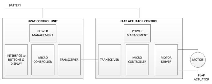
Figure 2. Remote Control of Flap Actuator Motor
