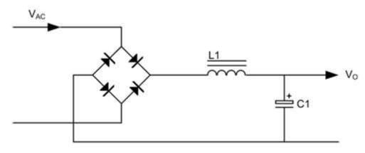
Figure 2. Typical Passive PFC with Inductor Compensation
