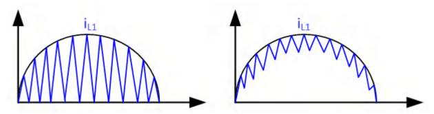
Figure 5. TM PFC (a); Continuous Conduction Mode PFC (b)
