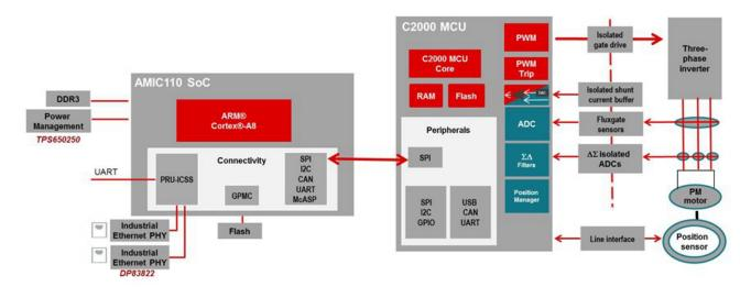
Figure 1. Example Implementation of Motor Control with AMIC110 and C2000
