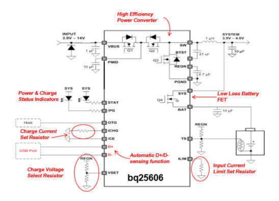
Figure 2. bq25606 Implementation Schematic
