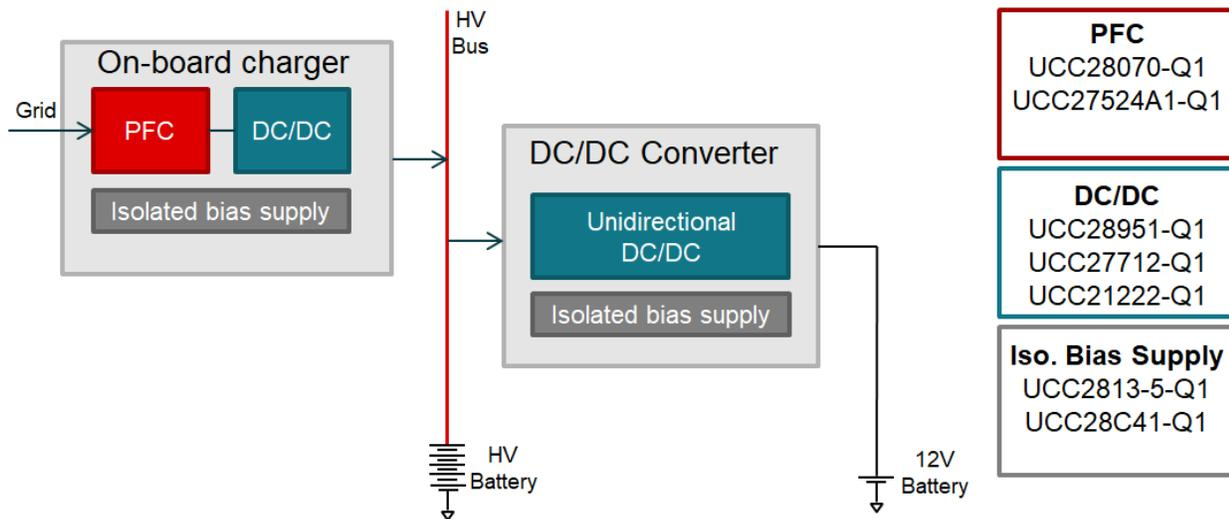
Figure 2. PFC and DC/DC Controller for On-board Charger
