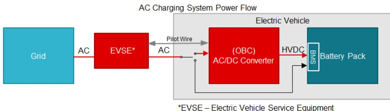
Figure 1. High Level System Block Diagram- On-board Charger
