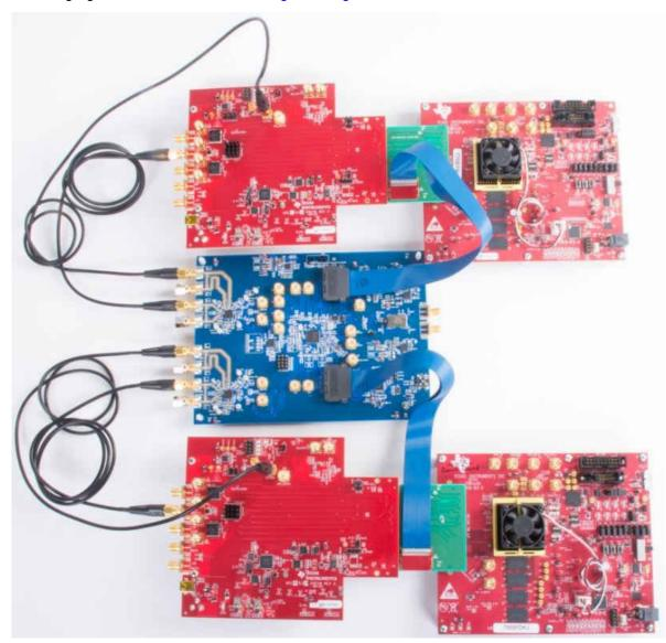
Figure 2. Channel-to-channel Skew Measurement Setup
