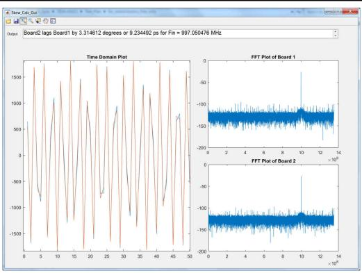
Figure 3. Measured Channel-to-channel Skew and Spectrum from Both Channels
