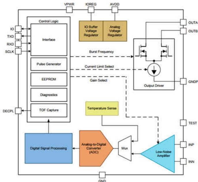
**Figure 4. PGA460 Functional Block Diagram**
