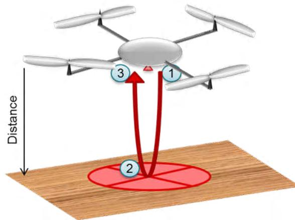
**Figure 2. Depiction of Ultrasonic ToF for Drone Landing**
