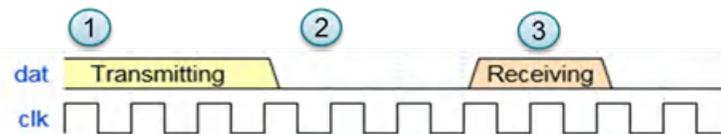
**Figure 3. Phases of Ultrasonic ToF**
