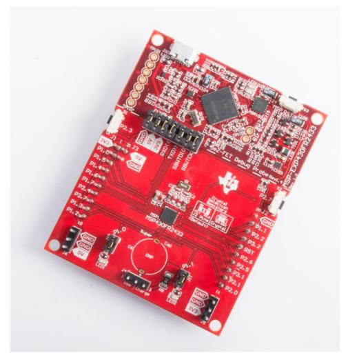
Using the 16-bit MSP430FR2433 microcontroller (MCU), the MSP-EXP430FR2433 is the latest LaunchPad kit supporting the MSP430™ value line sensing family. The MSP430FR2433 MCU features 16KB of memory with a 10-bit eight-channel analog-to-digital converter (ADC), four 16-bit timers, one I²C, two Serial Peripheral Interface (SPI) ports, two universal asynchronous receiver transmitters (UARTs) and a 32-bit hardware multiplier in a 4mm-by-4mm VQFN package.
