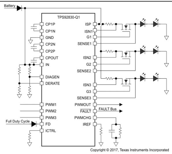
Figure 2. TPS92830-Q1 Simplified Schematic
