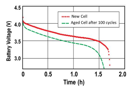
Figure 1. Effect of Cycling on Battery Performance
