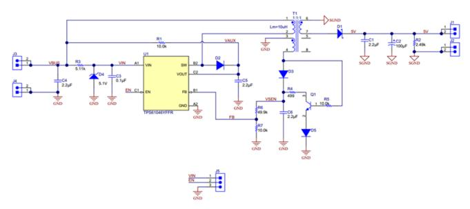
Figure 2. A Schematic of a Primary-side Regulation Flyback
