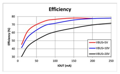
Figure 4. Efficiency at Different Input Voltages
