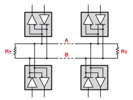
Figure 1. RS-485 Network Structure
