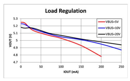
Figure 3. Load Regulation at Different Input Voltages
