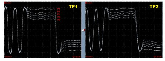
Figure 2. PCIe Tx Preset Family, before and after a Channel That Includes a Linear Equalizer
