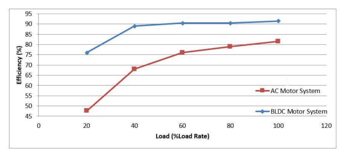
BLDC motors provide high efficiency. In addition, BLDC motors have long life and very low electric noise due to the lack of brushes, making them reliable for various applications such as appliances.
