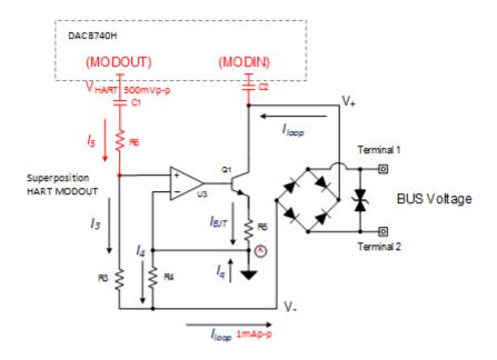
Figure 2. Superposition of HART Modem
