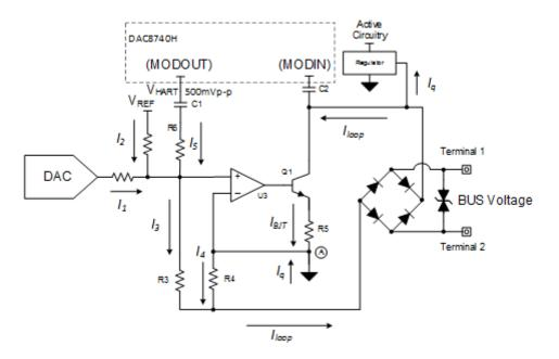
Figure 1. Two-wire Transmitter with HART Modem
