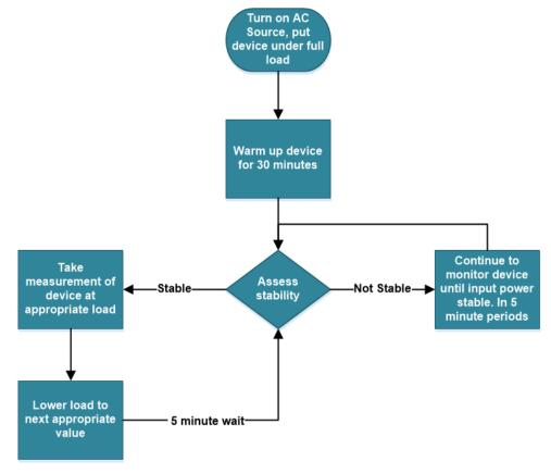
**Figure 3. Efficiency Measurement Procedure**
