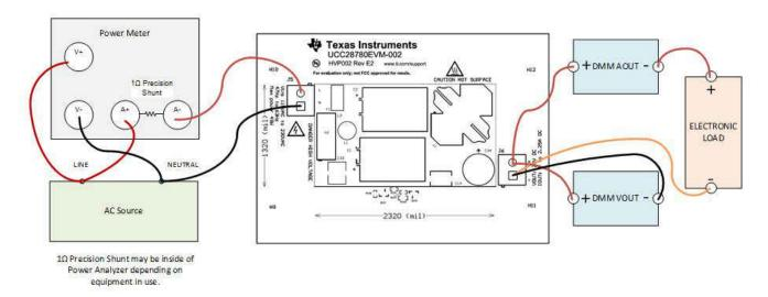
Figure 1. UCC28780EVM Connection Diagram for Efficiency Measurements
