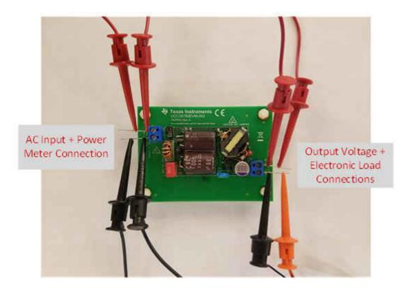
Figure 2. Probe Connections for Efficiency Measurements
