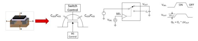
Figure 1. Switch Capacitance Structure
