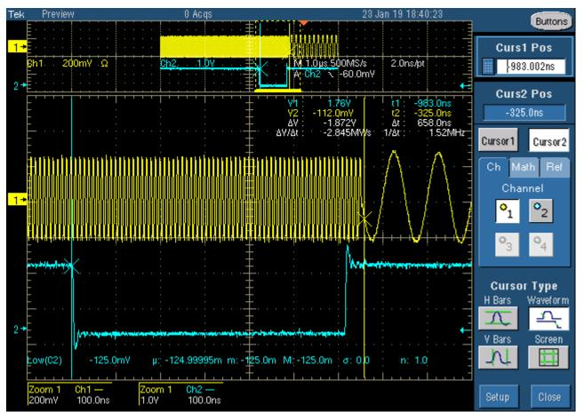
Figure 4. The Hop Time When Switching from One NCO to Another Is Approximately 660 Ns
