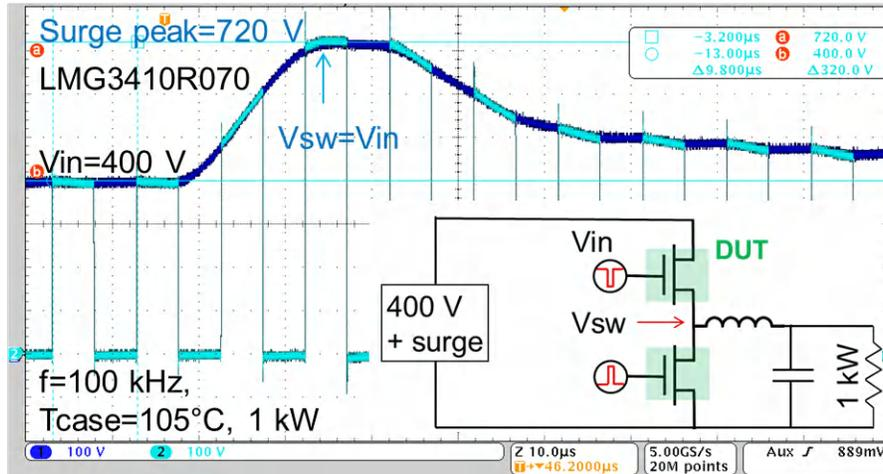
**Figure 2. Demonstration of the Surge Robustness of the LMG3410R070. the Input Bus Voltage Surges from the Operating Point of 400 v to the Target Specification of 720 v When the Active Circuit (Inset) Is Struck with a Surge Waveform Conforming to the IEC 61000-4-5 Standard. the Switched-node Waveform Is Overlaid on the Input Waveform to Show That the GaN FETs Successfully Switch through a 720-v Peak Bus Voltage Surge.**
