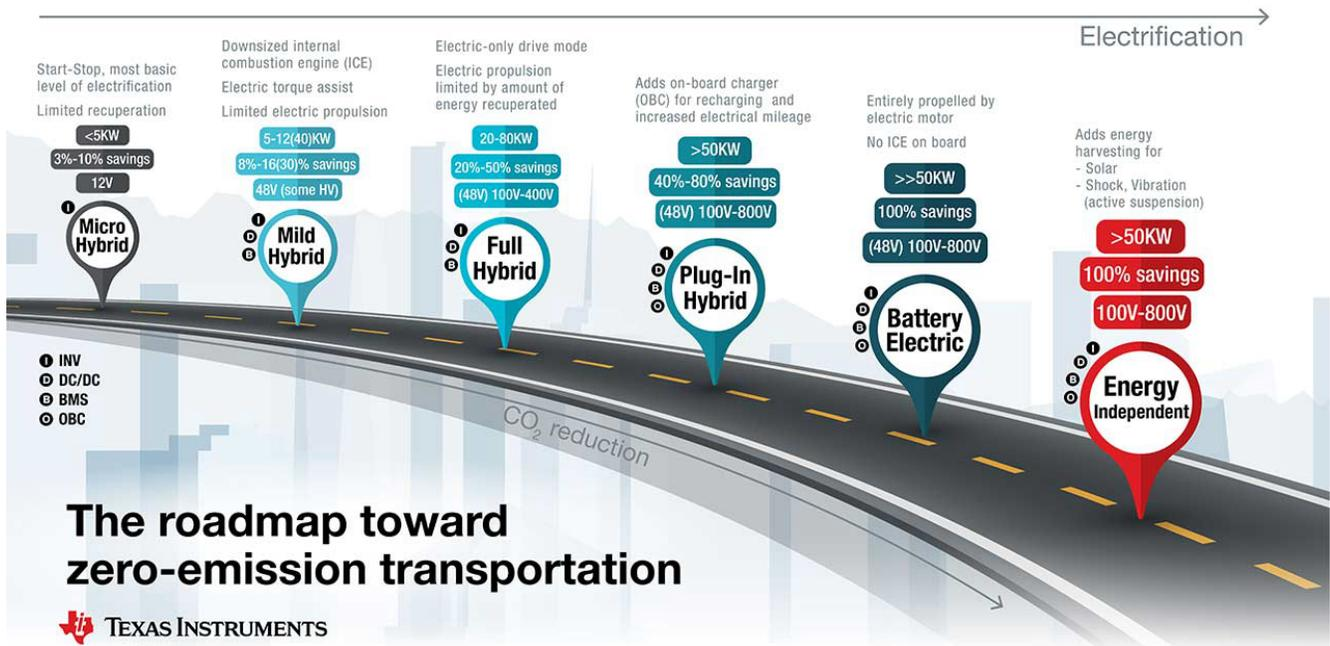
Figure 1. The Range of Hybrid to Electric Vehicles
