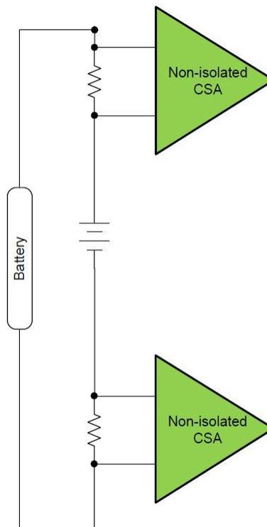
**Figure 1. Top of Stack vs. Bottom of Stack in a Battery Management System**
