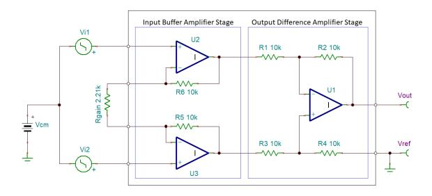
Figure 1. INA Internal Stage Diagram
