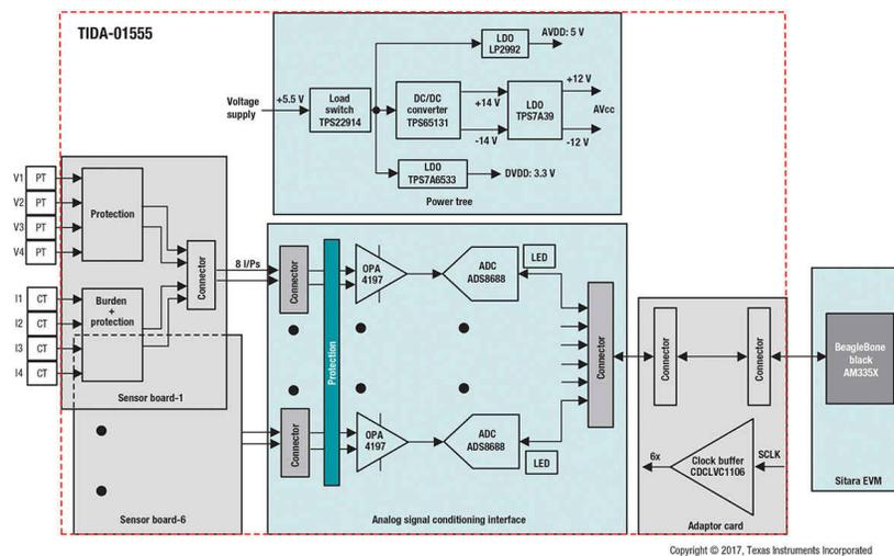
**Figure 2. Flexible Interface Reference Design Block Diagram**
