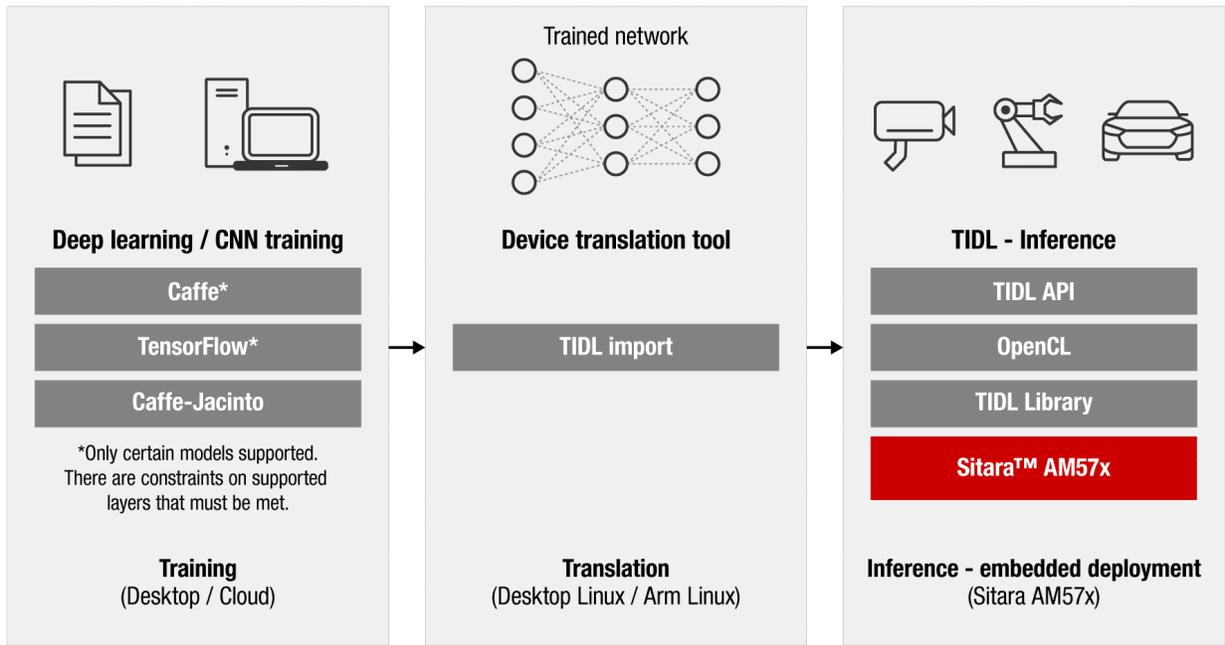
**Figure 3. TI Machine Learning Software Framework Process for the AM574x Processor**
