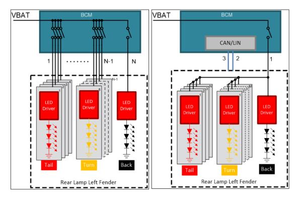
Figure 1-1. Traditional and new rear lamp architectures for pixel control
