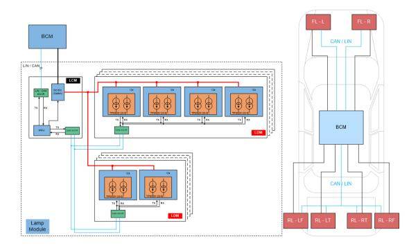
Figure 1-3. Typical application diagram for long-distance off-board communication
