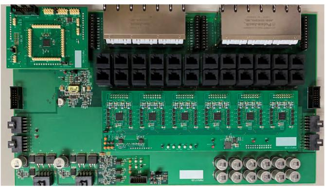
Figure 1-1. Evaluation board of TI's FirmPSE ecosystem
