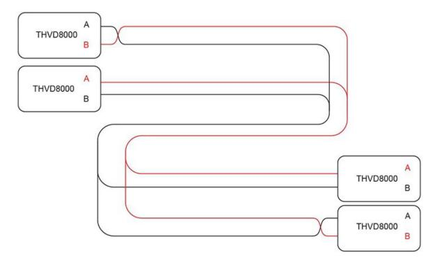
Figure 3. Polarity-free Mode with the THVD8000
