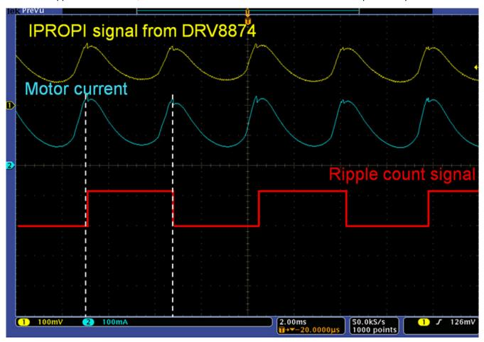
Figure 2. The IPROPI current feedback signal with ripples from brushed-DC motor commutation
