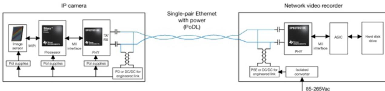
**Figure 2. PoDL example in video surveillance**
