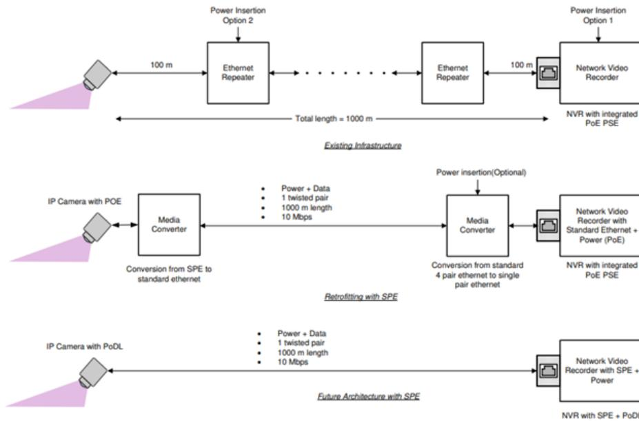
**Figure 3. IP network camera connectivity**
