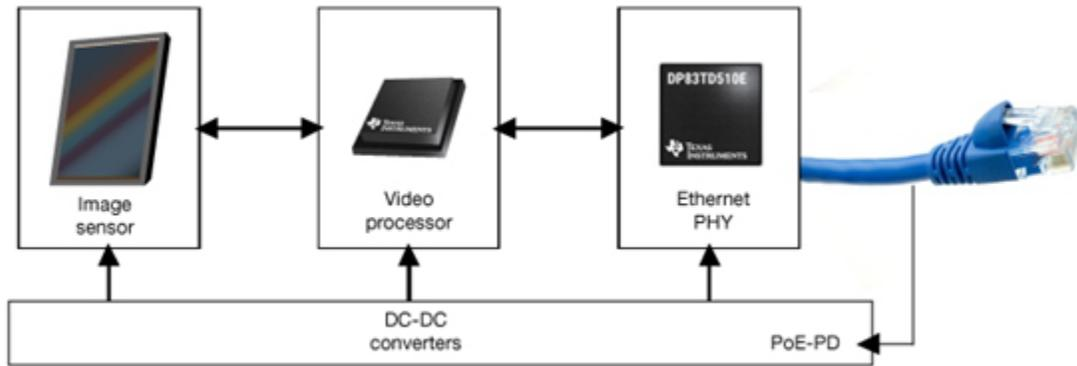
**Figure 1. A basic Internet Protocol (IP) surveillance camera**
